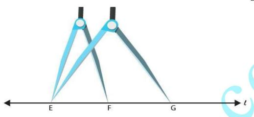
(ii) Construct a line I and mark a point E on it. Take a divider and open such that both its end arm are at A and B Lift the divider and place its one end at E and the other end as F on the line I
