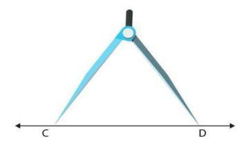
(v) In order to construct a line segment CD collinear with AB and is equal to it, use a ruler along AB and draw the line extended to AB. Take a divider and open it such that both of its end-points are the points A and B. Lift the divider and place its end-points of both of its arms on the extended line of AB and mark them as points C and D.
