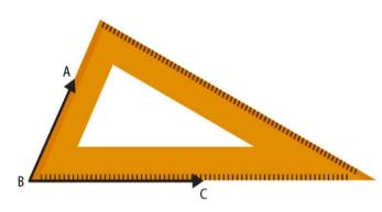
(iv) Now place 30° using set square and make an angle 60°. Construct two rays BA and BC as in given figure.
