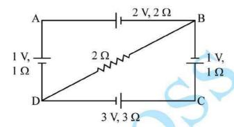
Using Kirchhoff's rules, calculate the potential difference between B and D in the circuit diagram as shown in the figure.
