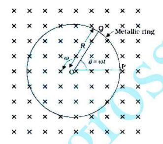
The magnitude of the emf, generated across a length dr of the rod, as it moves at right angles to the magnetic field, is given by
