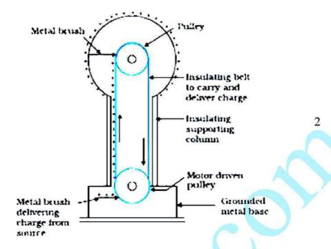
**Working:** The belt continuously carries positive charge, sprayed on to it by a brush at ground level, to the top. There it transfers its positive charge to another conducting brush connected to the large shell. Thus positive charge is transferred to the shell, where it spreads out uniformly on the outer surface. In this way voltage difference is built up.
