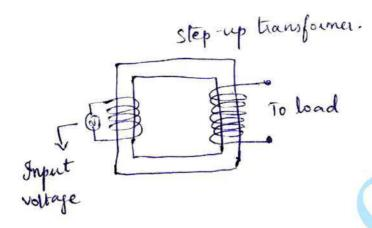
AC voltage  $v_i$  is applied at primary P of transformer (with turns  $N_P$ ).
