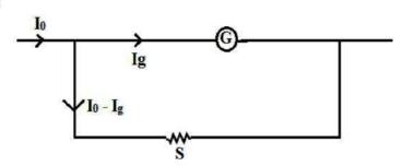
(G) can be converted into an ammeter by connected a small stunt resistance parallel to (G) coil so that
