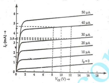
Output characteristics of an n-p-n transistor in CE configuration is shown in the figure. Determine:
